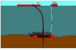
H. In order to stabilize the ship on the sea bottom and to neutralize the high oil pressure, heavy basalt blocks should be dumped through a shaft to the ship.
